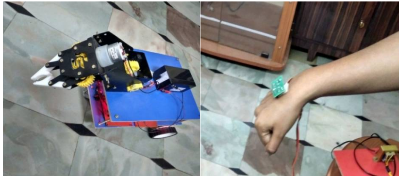
Fig MEMS used to move the Robot Arm downward direction
